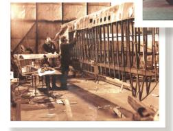
The wings were stripped down to its spruce wood spars and duralumin clad leading and trailing edges. Countless hours were spent removing glue or fabric and replacing small wooden parts which had decayed due to exposure.
