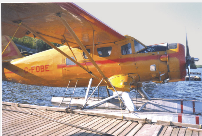
C-FOBE the world's only fully metalized Norseman at Green Airways shortly after it had been purchased by them and before it had been painted in their colours.
