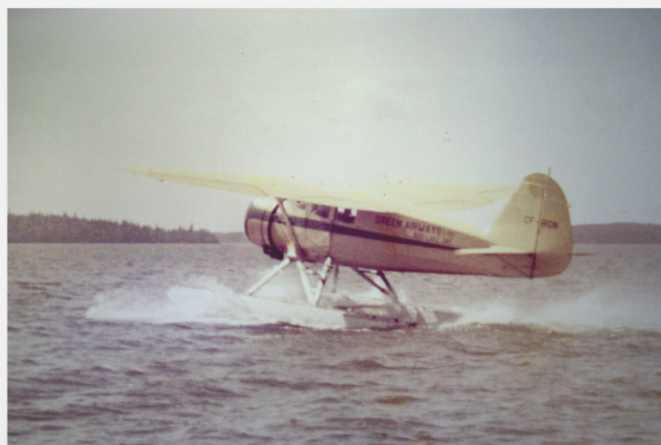
Green Airways Stinson Reliant Gullwing. The SR9s were originally produced with a 300 H.P. engine which left them underpowered. George Green put a P. & W. 450 H.P. Junior Wasp engine into the aircraft to solve the problem. To do so, he had to remake the original bubble cowling which would no longer fit over the larger engine.
